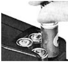
1. Load the batteries.
