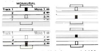
4-track monaural recording/playback sequence is 1-4-3-2. For monaural operation, depress LEFT Track Selector Switch. The first recording/playback takes place on track 1 and the second on track 4 after the recorder has been set to reverse mode. For recording/playback on track 3-2, depress RIGHT Track Selector Switch. The third recording/playback takes place on track 3 and the fourth on track 2 after the recorder has been set to reverse mode.
