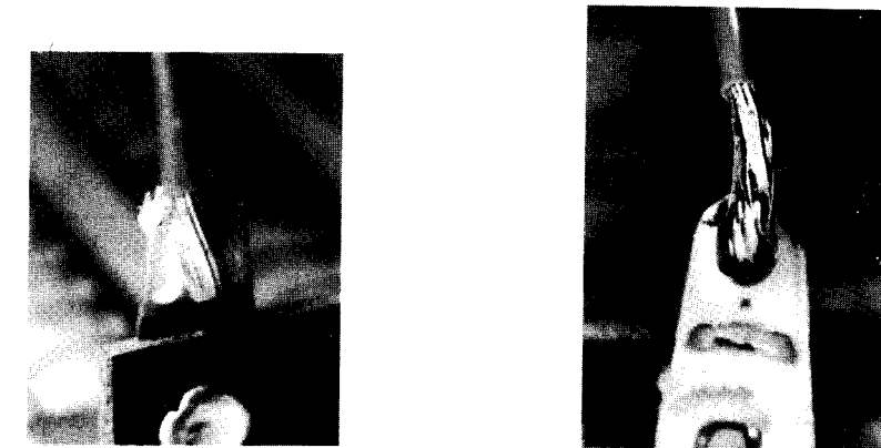
Fig. 7.8 Cold Solder Joint
