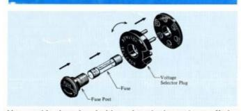
Your machine is equipped with a universal voltage selector offering six selections of voltage from 100V to 240V AC. Voltage is preset at the factory according to destination. However, the operator is requested to reconfirm setting and, if necessary, readjust as follows:
