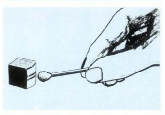
While GX Heads do not require a great deal of cleaning, if old tape which has been spliced, etc. is used, head cleaning is recommended. It is especially important that the heads be clean prior to recording. Remove head cover and clean the heads with a cotton swab stick which has been dipped in Akai Cleaning Fluid (from Head Cleaning Kit HC-500). Also clean the pinch roller, capstan shaft, and tape guides, etc. over which the tape travels.
