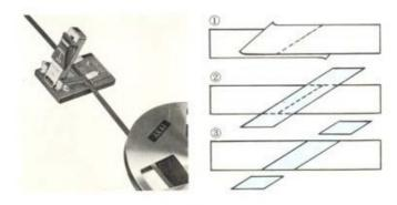
Cut tape diagonally with an overlap so that the ends are lined up (cutting on diagonal eliminates detection of splice in recording). Cover aligned ends with splicing tape. Press firmly exerting pressure to secure ends evenly. Trim off excess splicing tape, cutting into tape very slightly. This eliminates the possibility of a sticky splice. For smooth and easy tape splicing, Akai's portable tape splicer, Model AS-3 is recommended.
