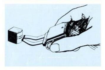
Normally, the steel pole pieces which form part of the recording and playback head become slightly magnetized. The effect of magnetization is considerable drop-out and noise. Therefore, it is recommended that head demagnetizing be performed periodically. This can be accomplished with a bulk Head Demagnetizer by bringing the prongs of the demagnetizer close to the heads and making several small circular motions over all head surface areas as well as the head housing.
